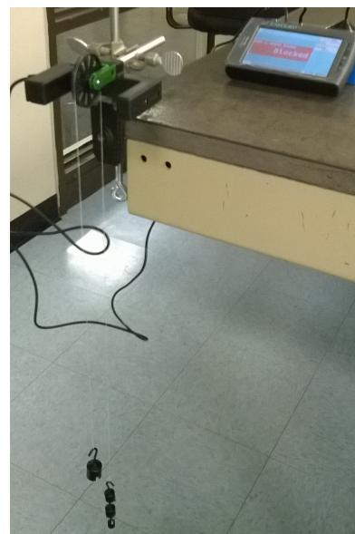
5. Release the system and stop it before the falling mass hits the ground (the other mass will hit the pulley if you do not stop the system).
